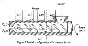
We divide the thermal barrel into four different temperature zones, as depicted in Figure 2, and analyze the thermal behavior in each zone separately. The thermal equation for each zone can be derived by the concept of thermal equilibrium of the system,
